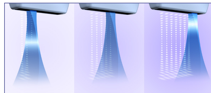
Figure 2. Linear Arrays, Multi-element Transducer. In order to create focused beams with these transducers a beamformer is required, which calculates the precise timing of excitation of each element. The combined effect of all the elements is a focused beam as illustrated.
